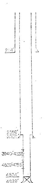
LEASE Florance WELL NO. 27A 9-5/8 "OD, 36 LB, K-55 CSG.W/ 225 SX TOC @ Surface 7 "OD, 23 L8, K-55 CSG.W/ 375 SX TOC @ Surface\_\_\_\_ 4-1/2 "OD. 10.5 LB, K-55 CSG.W/ 225 SX TOC @ 25591
