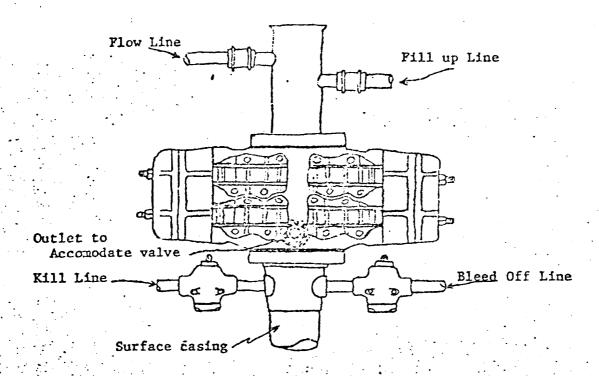
Blosout preventer is Shaffer double hydraulic equipped with drill pipe rams in the top and blind rams in the bottom.
