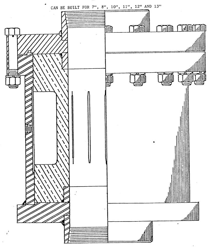
ADAPTER FLANGE - IS ESPECIALLY USEFUL IN LOCALITIES WHERE DEEP COLLARS ARE NOT AVAILABLE, AS IT WILL PROVIDE THE SHORTEST POSSIBLE HOOK - UP.
