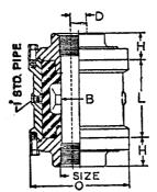
Model 3—Body assembled with Model 3 flanges (Blank or threaded). When the Blowout Preventer is assembled with Model 3 flanges at both ends, it presents the standard hook-up which may be placed in any position in the cellar by employing nipples of suitable length. Conventional practice in this hook-up, calls for a welded mud line connection, either above or below the Blowout Preventer.
