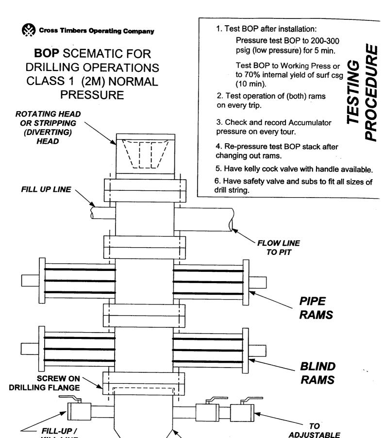
\*\* Remove check or ball from check valve and press test to same press as BOP's. \*\*
