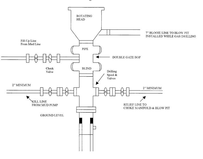
Minimum BOP installation for a Mesaverde well from Surface to Total Depth. 11' Bore, 2000 psi minimum working pressure double Gate BOP to be equipped with blind and pipe rams. A Schaffer Type 50 or equivalent rotating head to be installed on the top of The BOP. All equipment is 2000 psi working pressure or greater.
