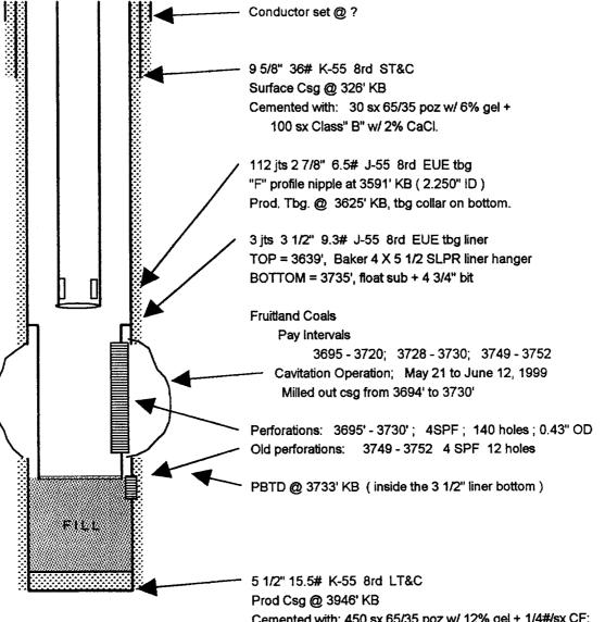
Cemented with: 450 sx 65/35 poz w/ 12% gel + 1/4#/sx CF; + 100 sx 50/50 poz w/ 2% gel + 6 1/4#/sx coal seal + 1/4#/sx cello-flake ( 1180 cu ft; 139 cu ft )
