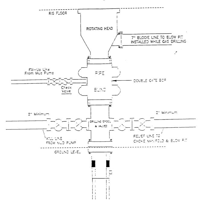
Minimum EOP installation for a Mesaverde well from Surface to Total Depth. 11" Eare, 2000psi minimum working pressure double gate EOP to be equipped with blind and pipe rams. A Schaffer Type 50 or equivalent rotating head to be installed on the top of the EOP. All equipment is 2000psi working pressure or greater.
