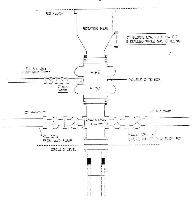
Minimum EOF installation for a Mesaverde well from Surface to Total Depth. 11" Eare, 2000psi minimum working pressure double gate EOF to be equipped with blind and pipe rams. A Schaffer Type 50 or equivalent rotating head to be installed on the top of the EOF. All equipment is 2000psi working pressure or greater.
