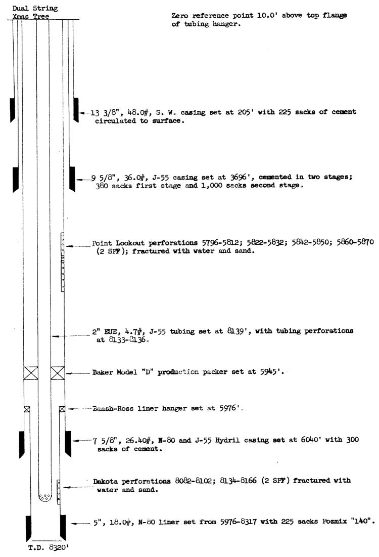
Note: Original 6 3/4" hole and two subsequent directional holes have fish in them and were plugged off. Hole containing liner drilled directionally from 6070' to Total Depth.
