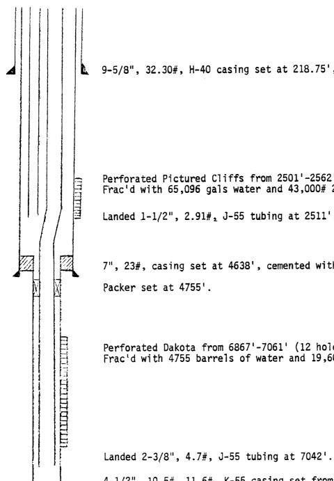
9-5/8", 32.30#, H-40 casing set at 218.75', cemented with 212 cu.ft. cmt.
