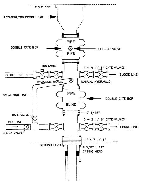
Minimum BOP installation for a typical open—hole Fruitland Cocl well from intermediate TD to TD. 7 1/16" Bore (6" Nominal), 2000psi working pressure/ or greater double stack double gate BOP equipped with three pipe and one blind ram.
