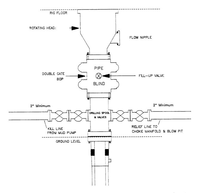
Minimum BOP installation for a typical Fruitland Coal well from surface to Intermediate casing point. 11" Bore (10" Nominal), 2000psi rninimum working pressure double gate BOP to be equipped with blind and pipe rams. A Schaffer Type 50 equivalent rotating head to be installed on the top of BOP. All equipment is 2000psi working pressure/or greater.
