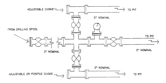
Minimum choke manifold installation for a typical Fruitland Coal well from surface to Total Depth. 2", 2000psi working pressure equipment with two chokes.
