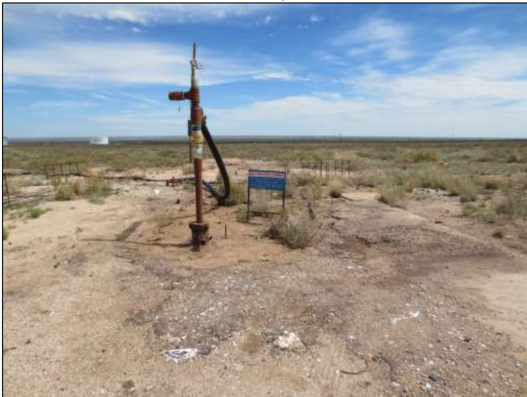
Well Head (Leak Source)
