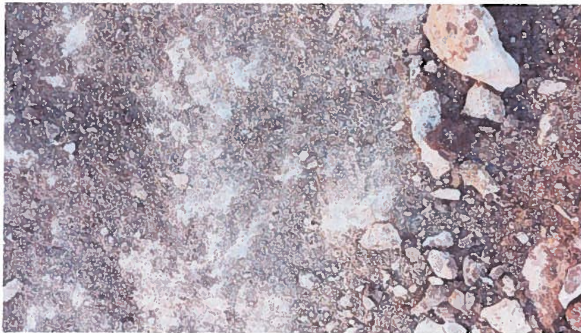
Figure 5. View looking down on hard-packed caliche layer that underlies the tank battery location at a depth of approximately three-feet below the ground surface.
