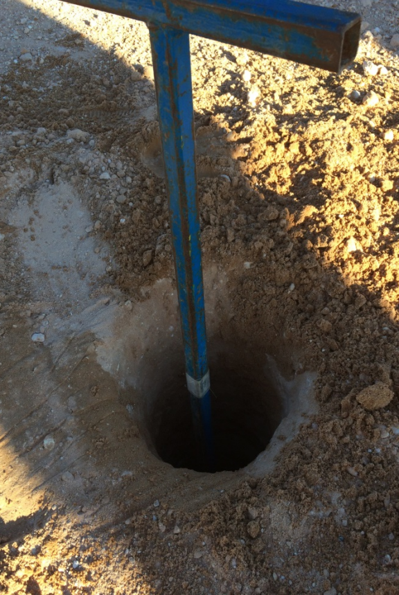
Collected 3 foot delineation samples in three locations around the tank battery
