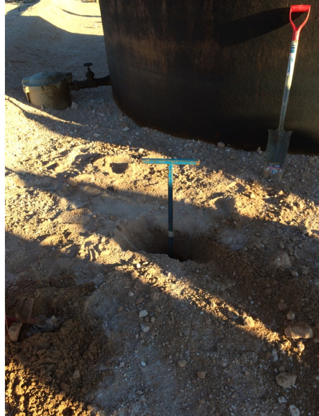
Collected 3 foot delineation samples in three locations around the tank battery
