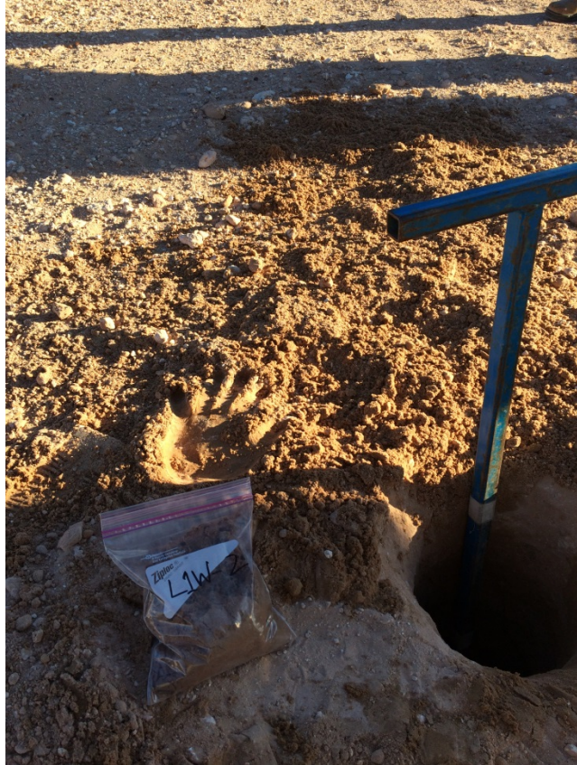
Collected 3 foot delineation samples in three locations around the tank battery
