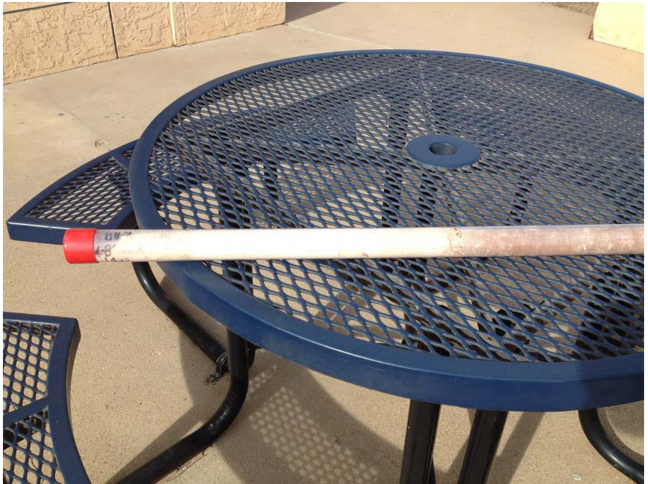
Figure 5. Core from 4 to 8 feet. Black cap is top of core, red is base. Sand at 4 feet grading to soft caliche at about 6 feet to base at 8 feet.
