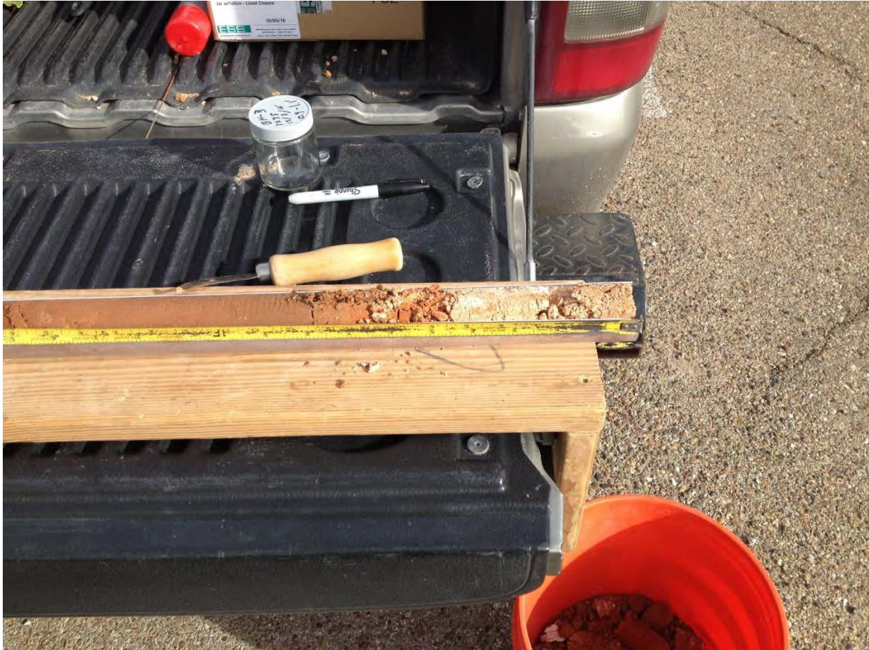
Figure 1. Borehole 3, top. White soil is mixture of sand and caliche at pad surface then a uniform fine-grained sand below. Soil sample for analysis to be taken at 1 foot (0.9-1.1 feet)
