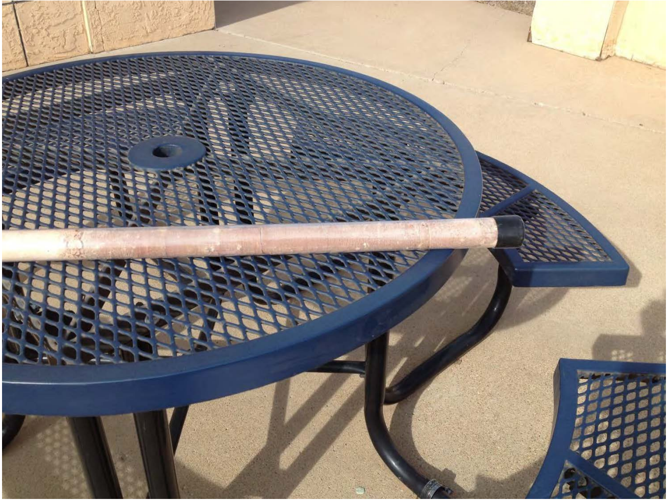
Figure 4. Core from 4 to 8 feet. Black cap is top of core, red is base. Sand at 4 feet grading to soft caliche at about 6 feet to base at 8 feet. Sample taken for analysis at 8 ft. Intermediate samples not to be tested unless sample at 4 feet shows contamination.
