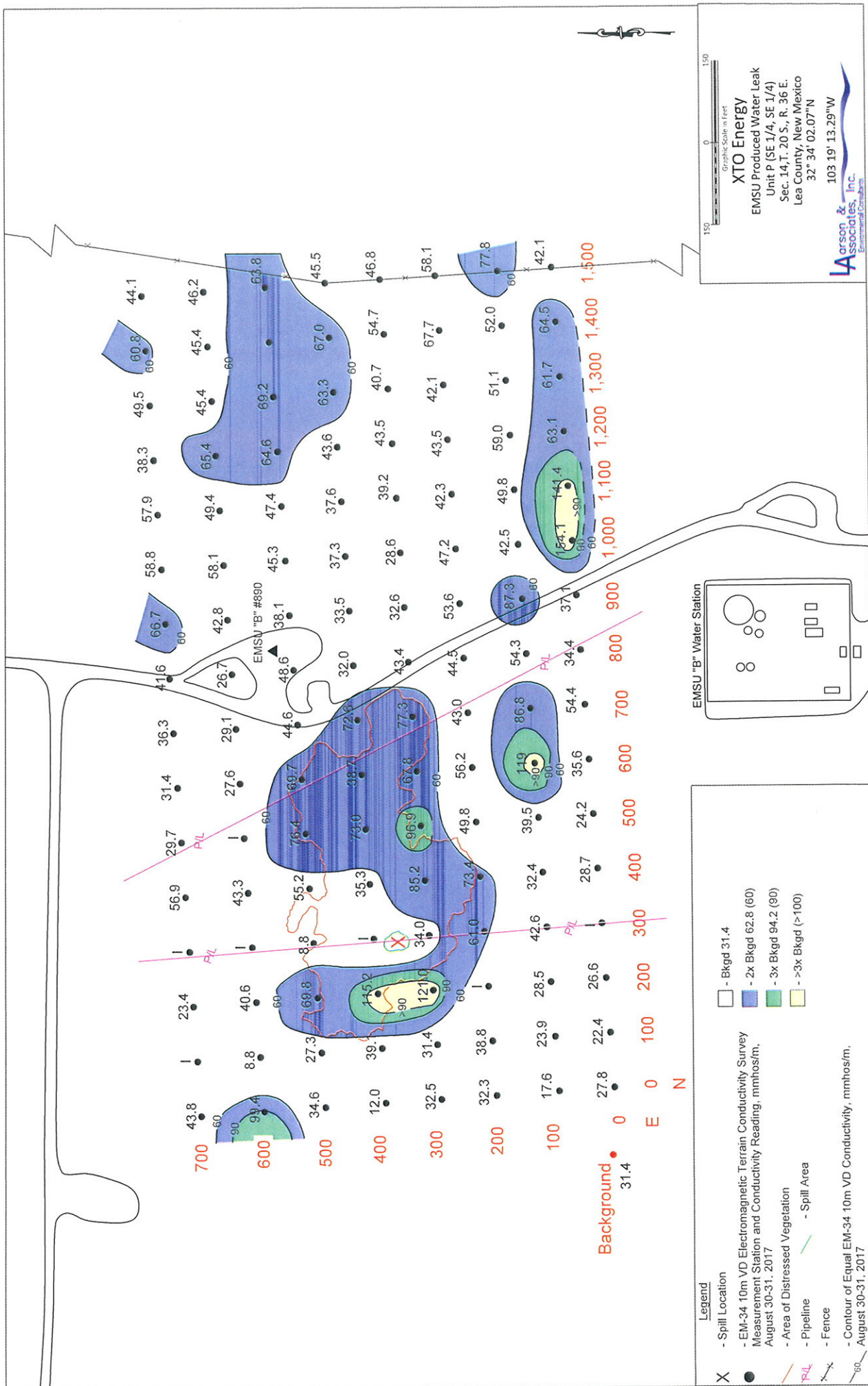
Figure 7 - EM-34 10m VD Conductivity Map, August 30-31, 2017
