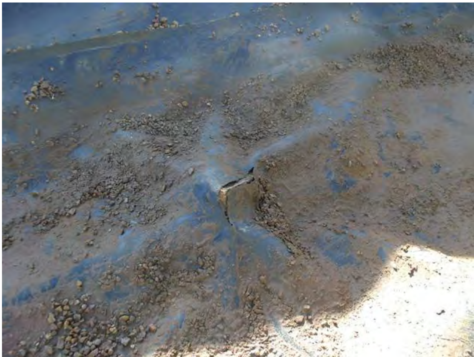
EPI Photograph Showing Tear in Liner, October 6, 2017
