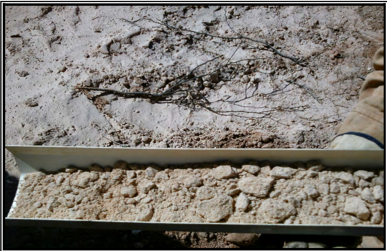
View of unindurated caliche sample after removal from plug sampler at Soil Boring 2.
