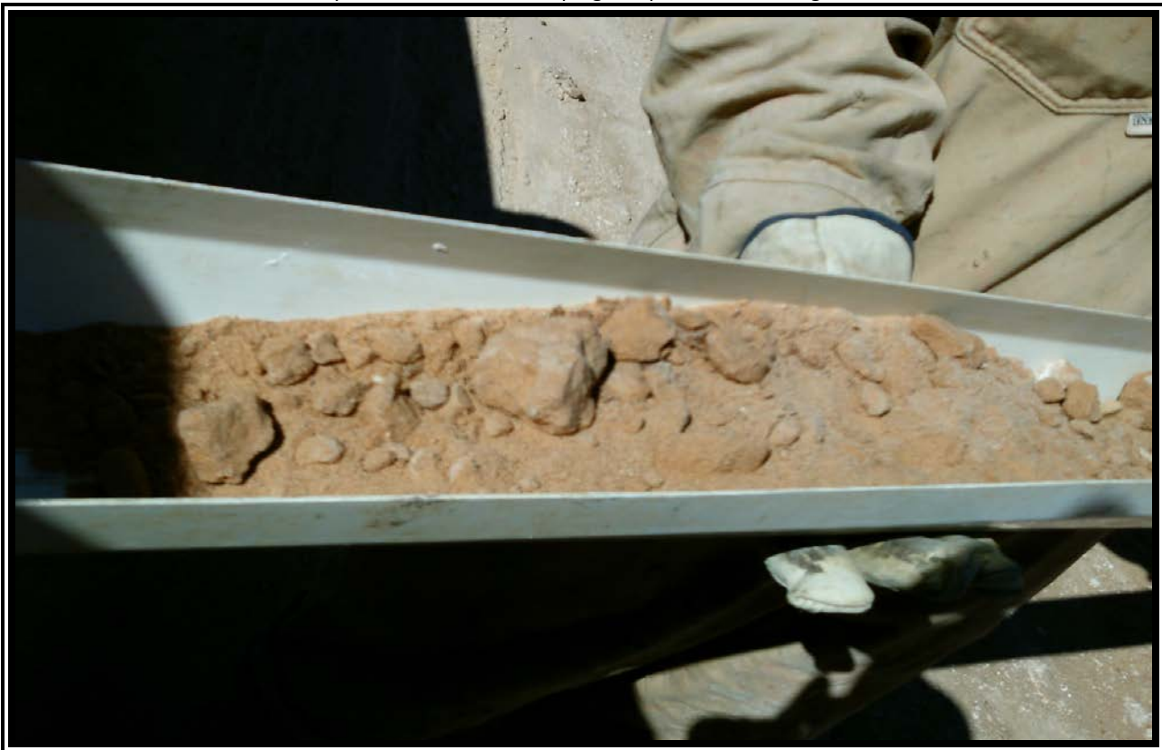
View of reddish tan fine grained sand sample after removal from plug sampler at Soil Boring 4.
