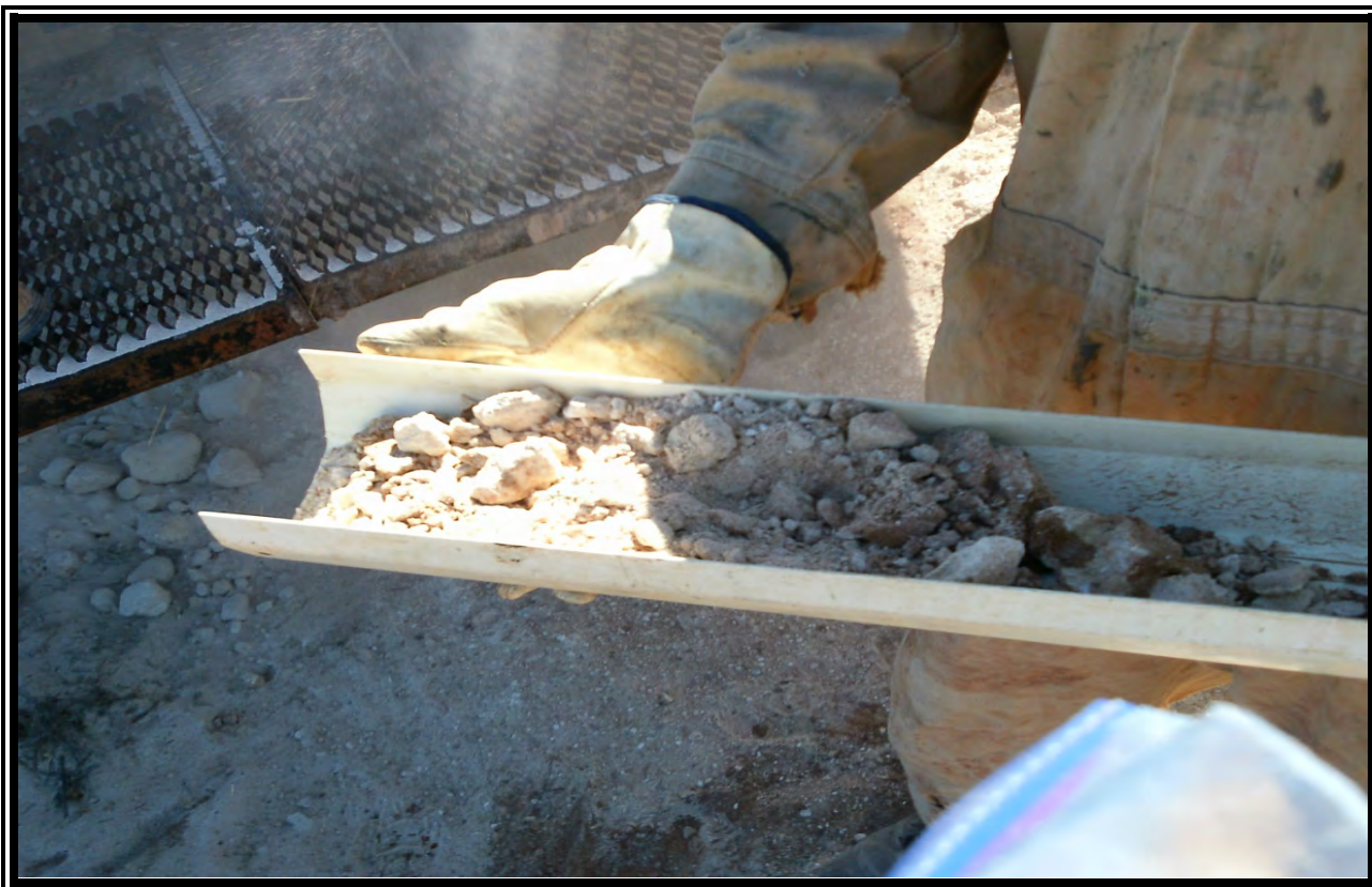
View of unindurated caliche sample after removal from plug sampler at Soil Boring 4.
