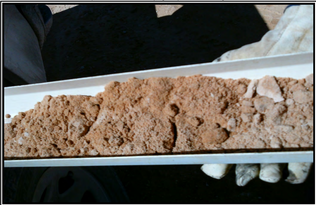
View of reddish tan fine grained sand sample after removal from plug sampler at Soil Boring 3.
