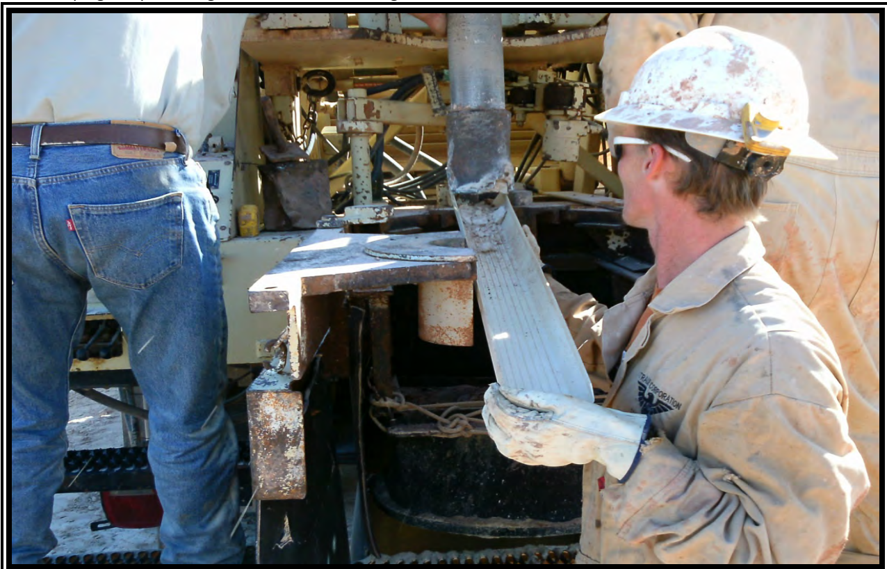
View of unindurated caliche sample being removed from plug sampler at Soil Boring 4.
