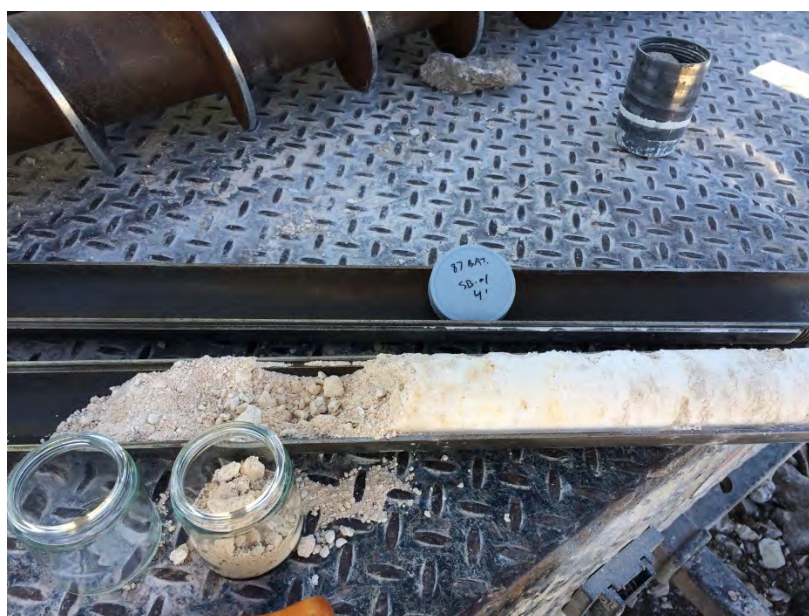
Exhibit F: SB-01 2017 split-spoon core sampling at 4-feet. Core sample is from 4-feet (left) to 6-feet (right). Caliche dominates the core sample.
