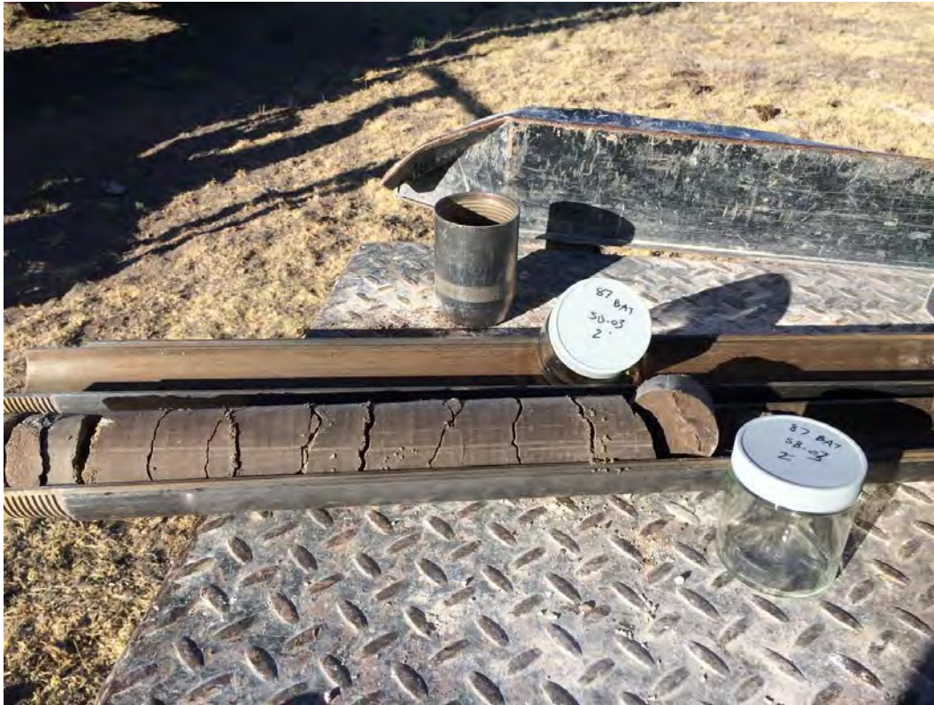
Exhibit D: Split spoon sample core at SB-03 Playa. 0-feet is at left. 2-feet is at right. Silty sand dominates the upper soil column from the surface to 6-feet.
