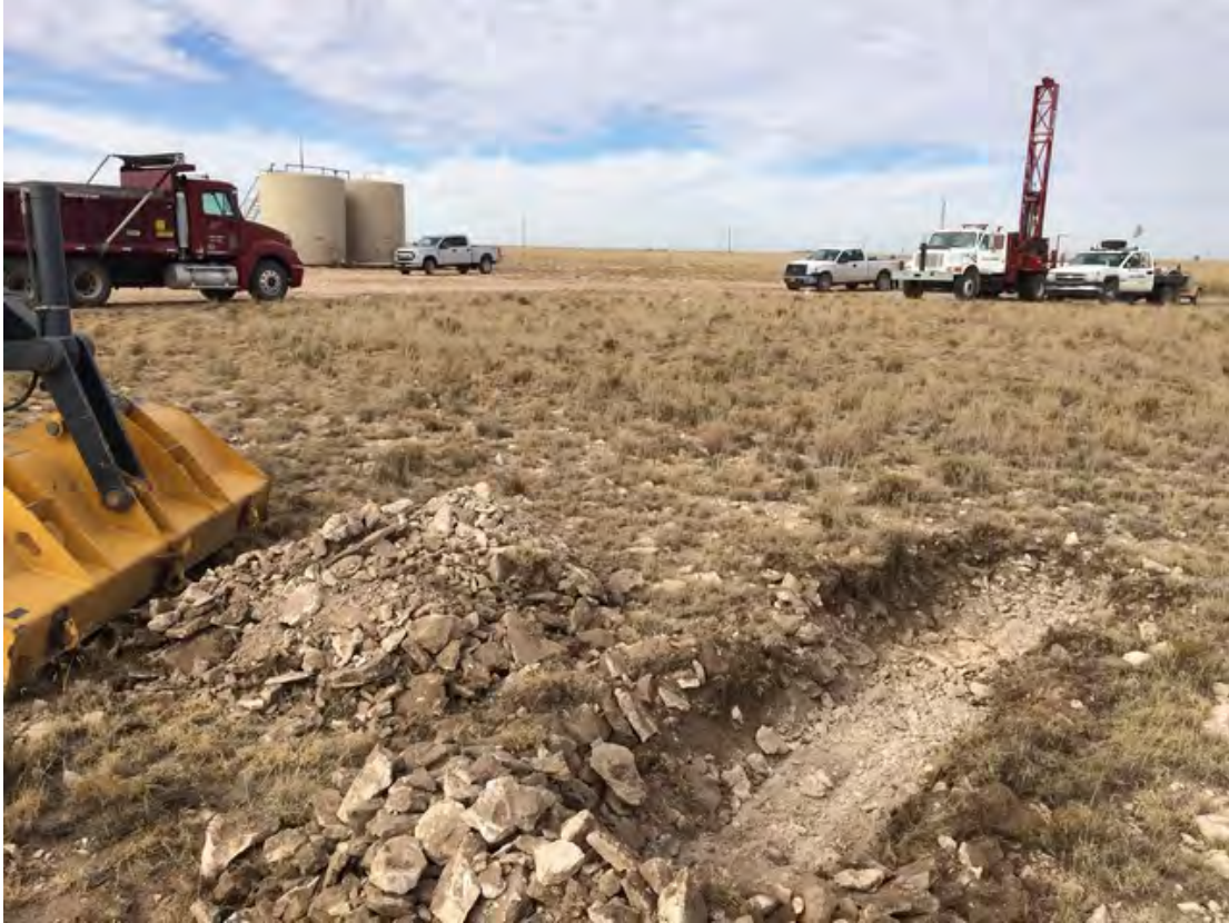
Exhibit B: Trench sample at Historic Southeast. Hard caliche encountered at 1-foot below ground surface. Land surface is undergoing natural restoration/re-vegetation. Drilling of SB-02 is visible in upper right of photo.
