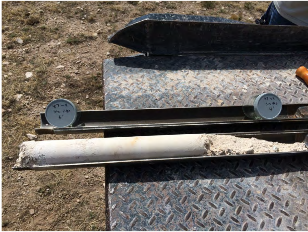
Exhibit G: Split-spoon core from 4-feet (right) to 6-feet (left) at SW Pad. Caliche dominates the core sample.
