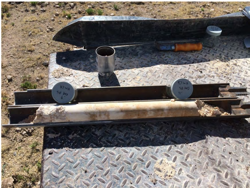
Exhibit E: Split-spoon core from 4-feet (right) to 6-feet (left) at SE Pad. Caliche dominates the core sample.
