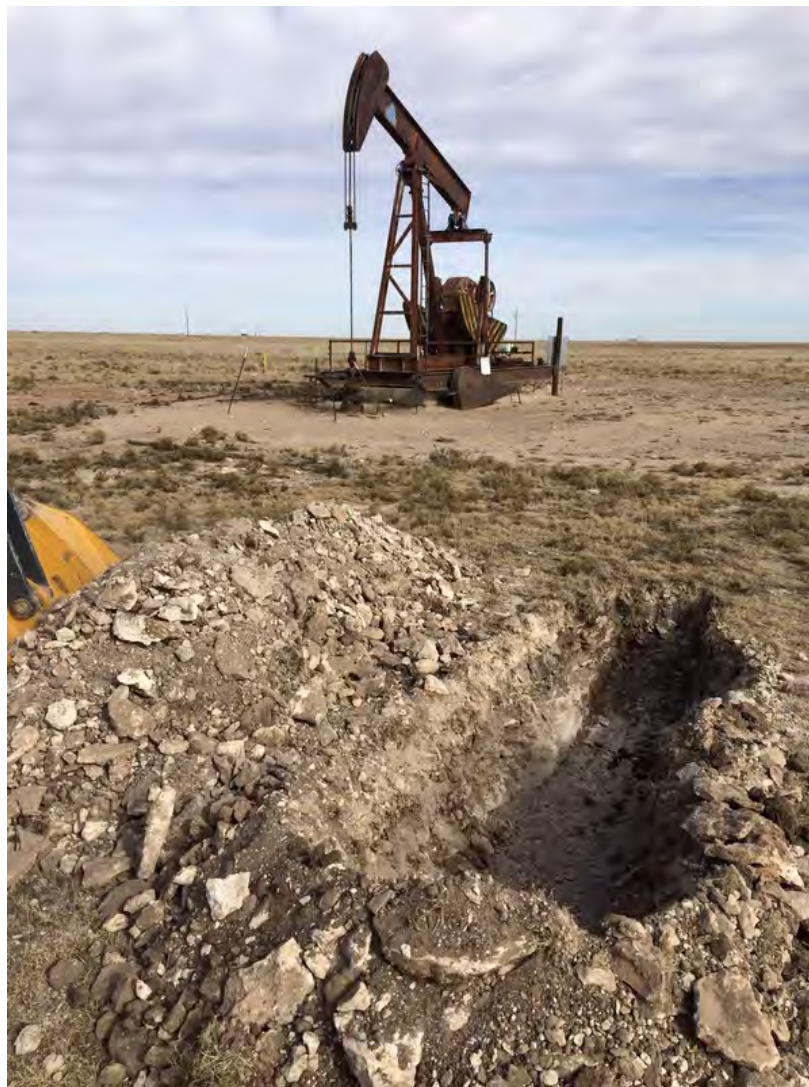
Exhibit B: Trench sample at SW Pad. Hard caliche encountered at 1-foot below ground surface. Total depth was 2-feet below ground surface. Land surface is undergoing natural restoration/re-vegetation.
