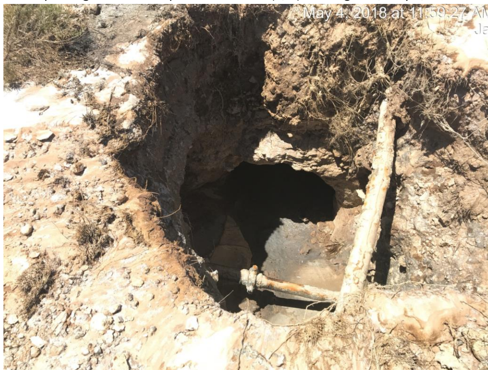
Washout from Injection Line Rupture East of Cooper Jal Unit #222 (P/A), May 4, 2018
