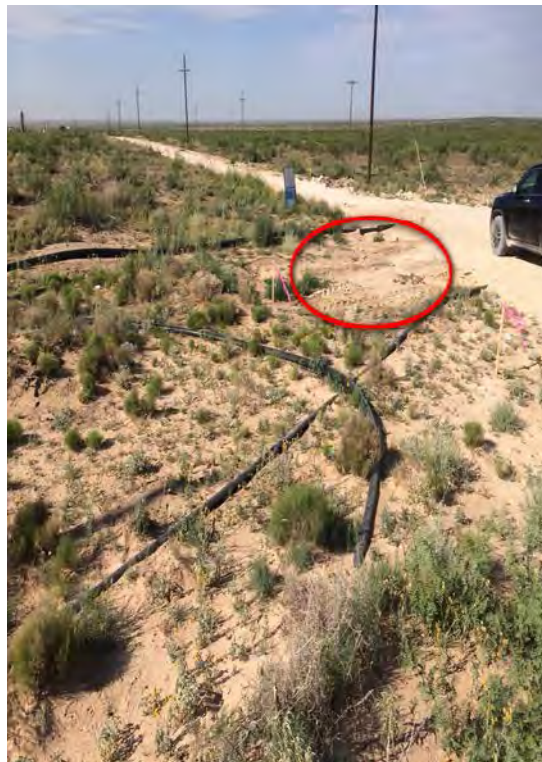
Figure M 1: Photograph viewing south along access road. The red circle is a potential location for one borehole for vertical delineation that is within the spill release area. The remaining spill area is undergoing natural revegetation. Numerous on-surface flowlines cross the area.
