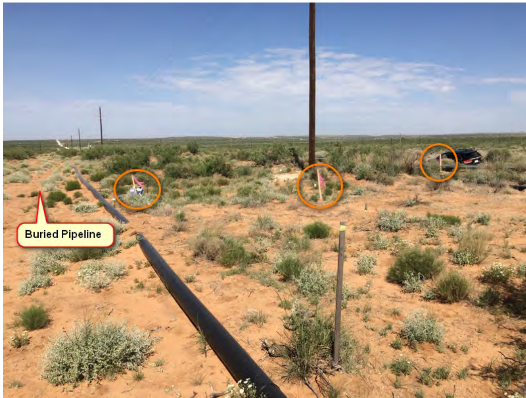
Figure M 4: Photograph viewing west along powerline/pipelines. Powerlines and flowlines restrict access to drill rig. Proposed boreholes are identified with pink flagging (see orange circles). From left to right : 32 26 50 South, 32 26 50 East, and 32 26 50 Pooling.
