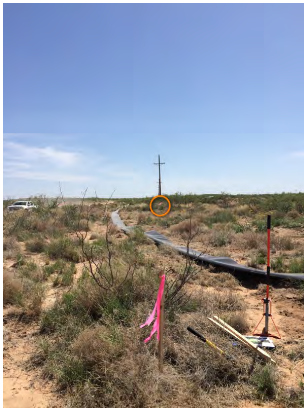
Figure M 3: Photograph at E. of Battle 34, viewing east. Proposed boring Southwest (foreground) and Southeast (background, orange circle) are identified by pink flagging. Powerlines are directly overhead. Drill rig requires 20-feet of clearance from powerlines.
