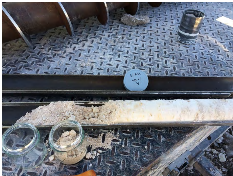
Exhibit F: SB-01 2017 split-spoon core sampling at 4-feet. Core sample is from 4-feet (left) to 6-feet (right). Caliche dominates the core sample.
