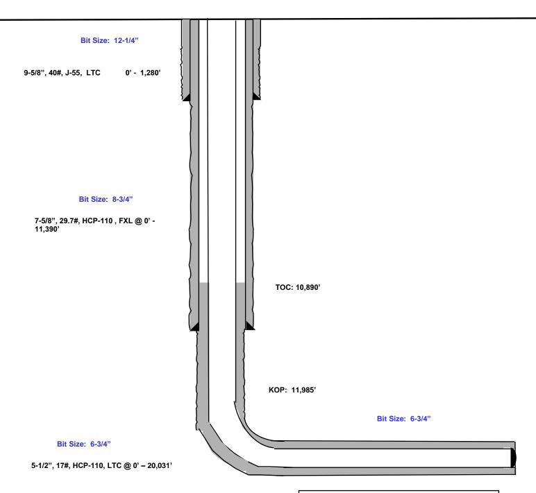
Lateral: 20,031' MD, 12,455' TVD BH Location: 2540' FNL & 330' FWL Section 32 T-24-S, R-33-E 374' FNL 554' FWL Section 29 T-24-S, R-33-E
