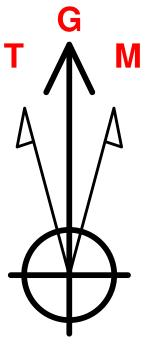
Azimuths to Grid North True North: -0.44° Magnetic North: 6.23°
