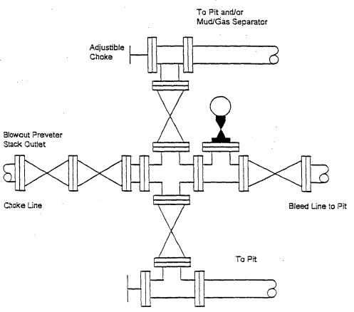
Flow Line R-Blind Rams **R-Pipe Rams** Drilling Spool Choke Manifold
