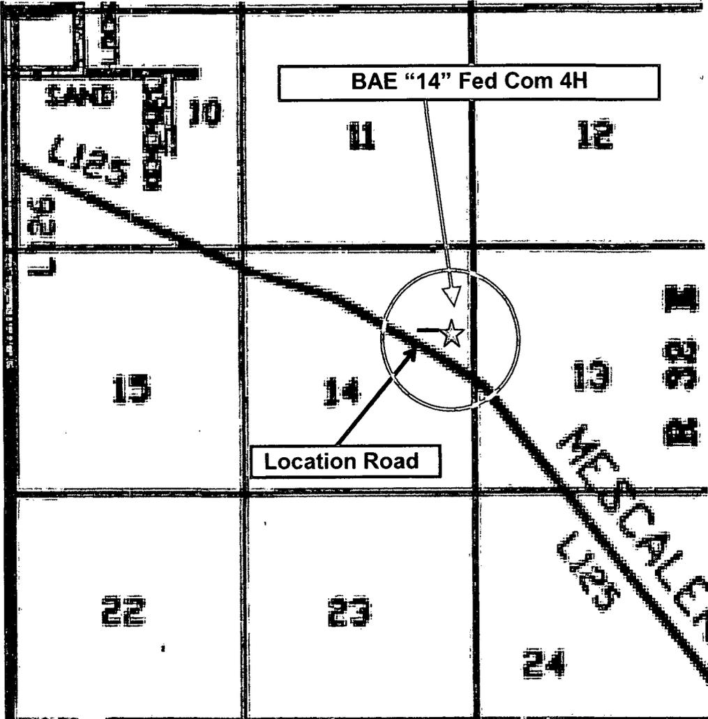
Assumed 100 ppm H<sub>2</sub>S concentration shall trigger activation of this plan. 3000' (Radius of Protection)
