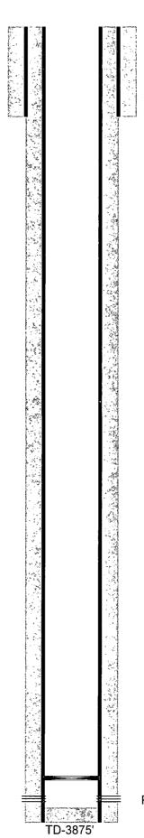
12-1/4" hole @ 424' 8-5/8" csg @ 424' w/ 350sx-TOC-Surf-Circ
