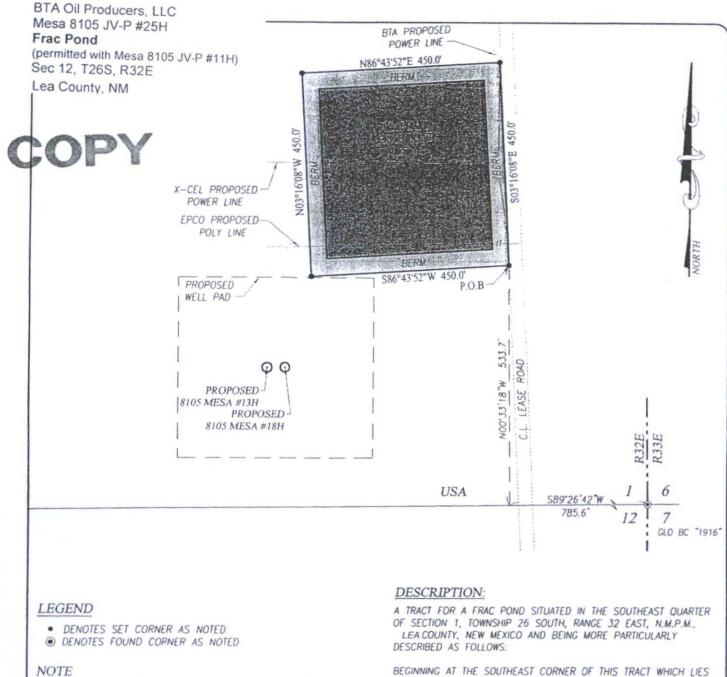
BEARINGS SHOWN HEREON ARE MERCATOR GRID AND CONFORM TO THE NEW MEXICO COORDINATE SYSTEM "NEW MEXICO EAST ZONE" NORTH AMERICAN DATUM 1983, DISTANCES ARE SURFACE VALUES.
