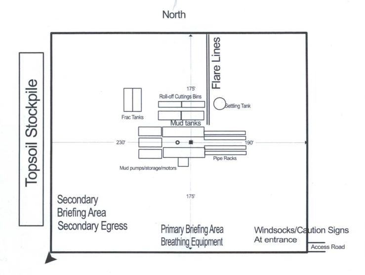
Alarms will be placed on the mud tanks, at the shale shaker, and on the rig floor. Windsocks will also be present on the top of the substructure and near the mud tanks.
