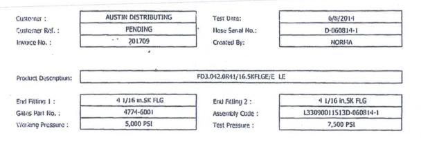
Gates E & S North America, Inc. certifies that the following hose assembly has been tested to the Gates Oilfield Roughneck Agreement/Specification requirements and passed the 15 minute hydrostatic test per API Spec 7K/Q1, Fifth Edition, June 2010, Test pressure 9.6.7 and per Table 9 to 7,500 psi in accordance with this product number. Hose burst pressure 9.6.7.2 exceeds the minimum of 2.5 times the working pressure per Table 9.
