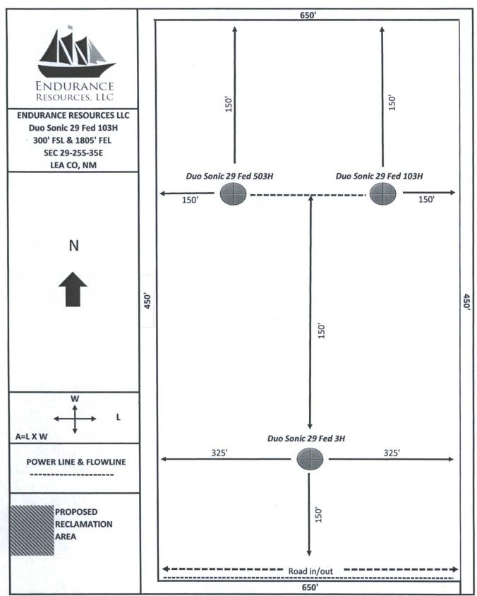
BLM has authorized multi-well (2 and 3 well pads) in lieu of single well pads, in conjunction with a centralized tank battery for the Duo Sonic 29 Fed productive wells. No reclamation is proposed at this time. Tank battery and wellsite will be constructed as needed by operations.
