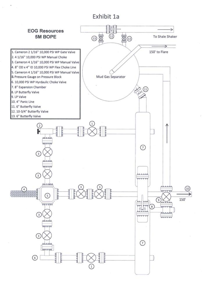
EOG 5M Choke Manifold Diagram (rev. 3/21/14)
