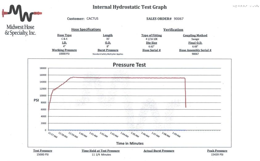
Comments: Hose assembly pressure tested with water at ambient temperature.
