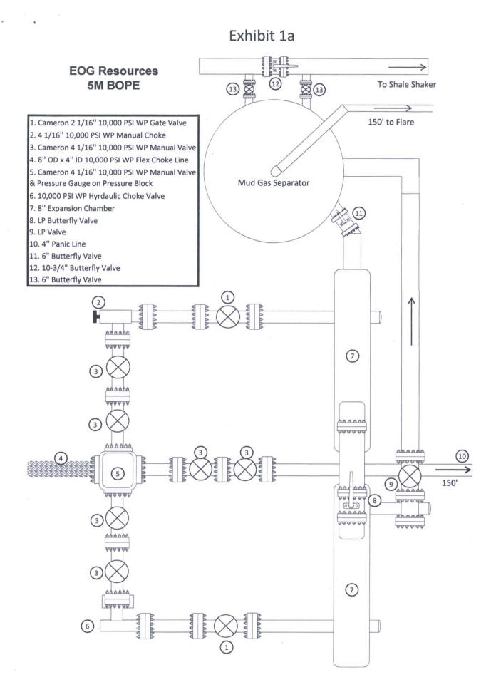
EOG 5M Choke Manifold Diagram (rev. 3/21/14)
