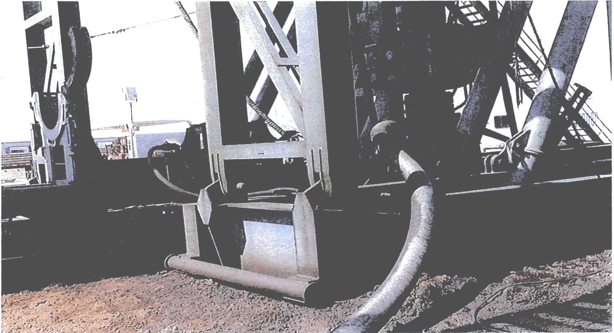
Exhibit F – Co-Flex Hose Triste Draw 25 Federal Com 14H Cimarex Energy Co. 25-23S-32E Lea County, NM
