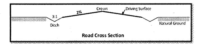
f. The access road will be constructed with a ditch on each side of the road.
