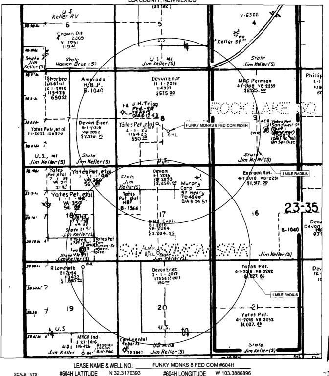
ALL BEARINGS, DISTANCES, AND COORDINATE VALUES CONTAINED HEREON ARE GRID BASED UPON THE NEW MEXICO COORDINATE SYSTEM OF 1983, EAST ZONE, U.S. SURVEY
