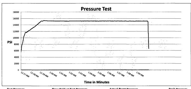
Test Pressure 15000 PSI Time Held at Test Pressure
