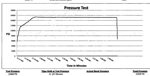
Comments: Hose assembly pressure tested with water at ambient temperature.
