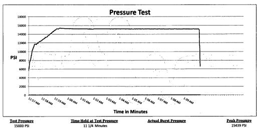
Comments: Hose assembly pressure tested with water at ambient temperature.
