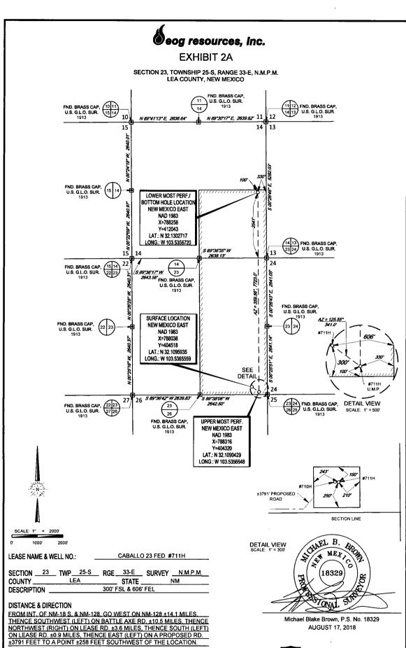
ALL BEARINGS, DISTANCES, AND COORDINATE VALUES CONTAINED HEREON ARE GRID BASED UPON THE NEW MEXICO COORDINATE SYSTEM OF 1983, EAST ZONE, U.S. SURVEY FEET.
