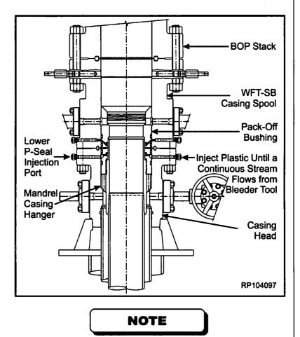
The strength of a mandrel casing hanger slick neck is equivalent to P110 Grade casing with the same weight as run in the casing string.
