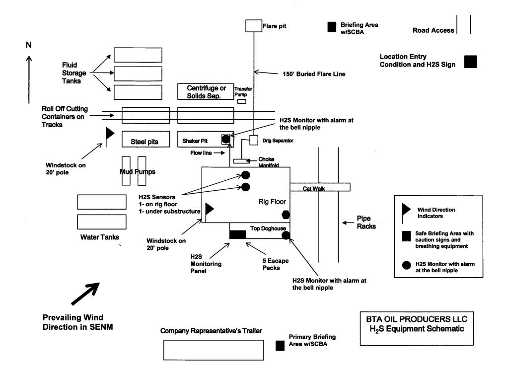
2 - portable H2S monitor positioned on location for best coverage and response. These units have warning lights and audible sirens when H2S levels of 20 ppm are reached.
