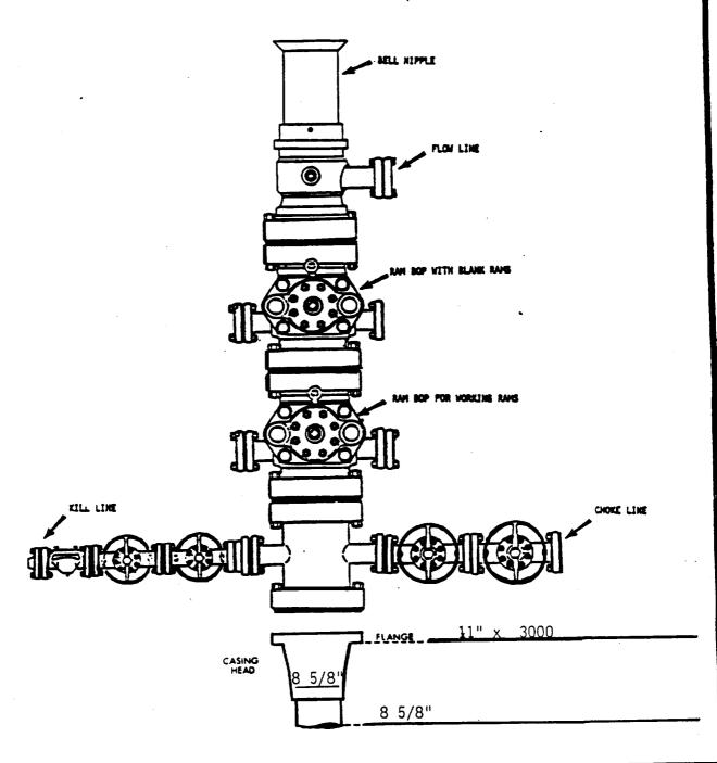
\*NOTE: ALL VALVES ARE METAL-TO-METAL SEAL AND FLAMGED.
