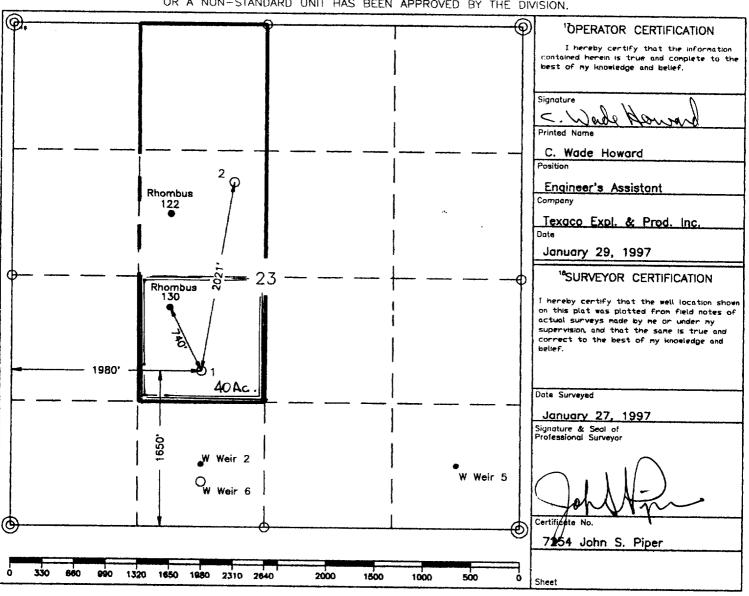
O = Staked Location • = Producing Well = Injection Well  $\diamond$  = Water Supply Well + = Plugged & Abandon Well
