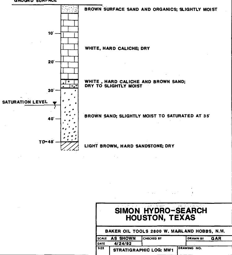
GROUND SURFACE BROWN SURFACE SAND AND ORGANICS; SLIGHTLY MOIST 10' -WHITE, HARD CALICHE; DRY 20' WHITE, HARD CALICHE AND BROWN SAND; DRY TO SLIGHTLY MOIST 30' SATURATION LEVEL BROWN SAND; SLIGHTLY MOIST TO SATURATED AT 33' 40' -TD=48 LIGHT BROWN, HARD SANDSTONE; DRY
