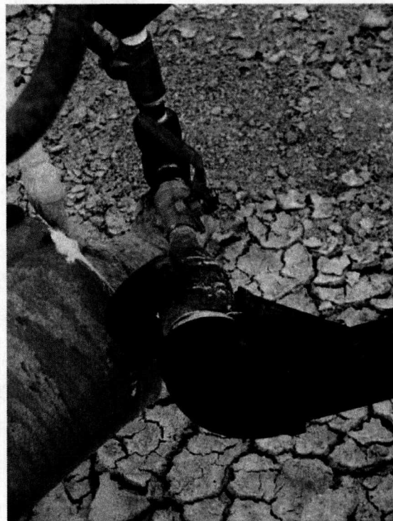
Recommended AFE to replace ½ inch dia. pipe with 1 inch or greater.
