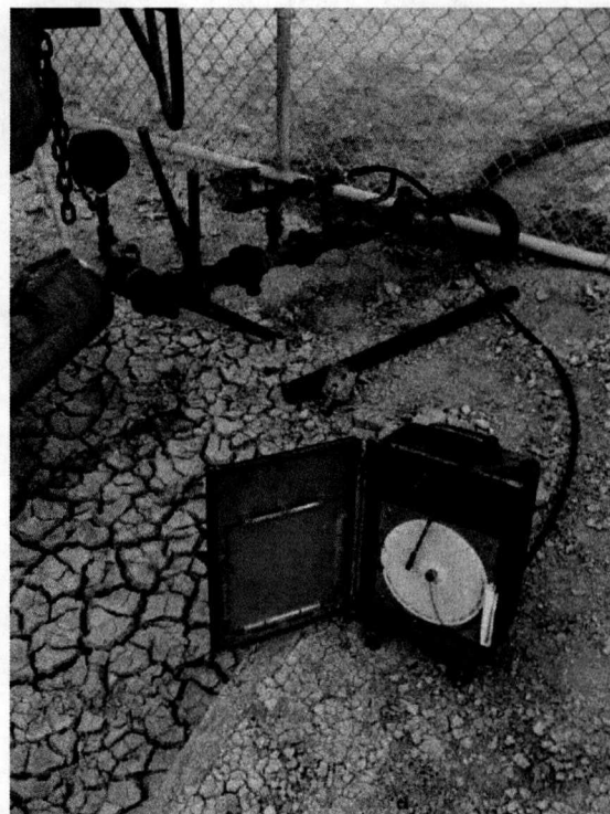
Chart recorder setup w/ valve arrangement during MIT
