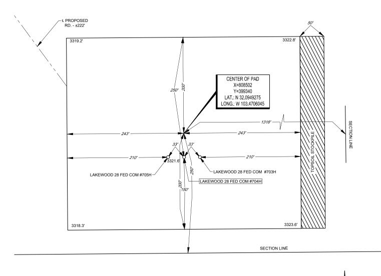
LEASE NAME & WELL NO.: \_\_\_\_\_ LAKEWOOD 28 FED COM #704H #704H LATITUDE N 32.0947908 \_\_\_\_ #704H LONGITUDE W 103.4706051
